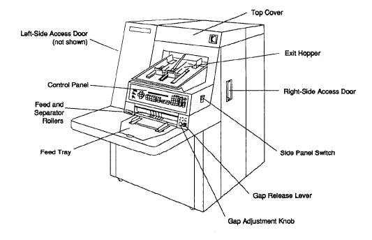
Control Panel – contains the Status Display, Indicators, and Operating Keys used to control the Scanner.
